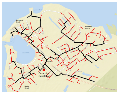
Figure 3 - Ocracoke Substation circuit map.
